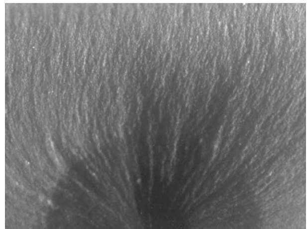
Fig. 4. A fracture surface from which the aspect ratio was measured. The semi-ellipse is visible because the sub-critical crack growth is transgranular, while the super-critical crack growth is intergranular. When light is parallel to the fracture surface, the semi-ellipse becomes visible.
